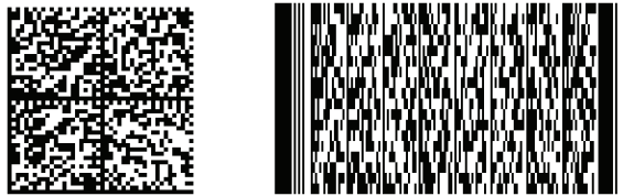
Illustration 1 – Datamatrix Code and PDF417 Code
